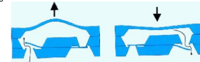
Fig. 6.1. Working principle of displacement pumps, in this case with two valve rectifiers (JD: ask Roland for source)
